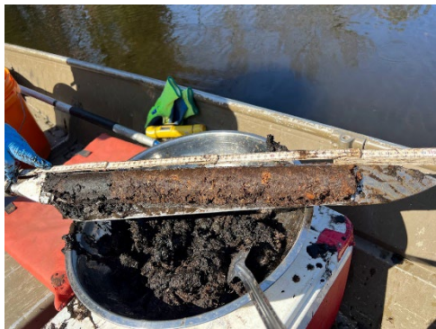
Sediment Core Sample from Dufresne Pond. A thick (>1 foot) layer of accumulated organic material (e.g., roots and dead plants) makes up the top layer of soft sediment.
